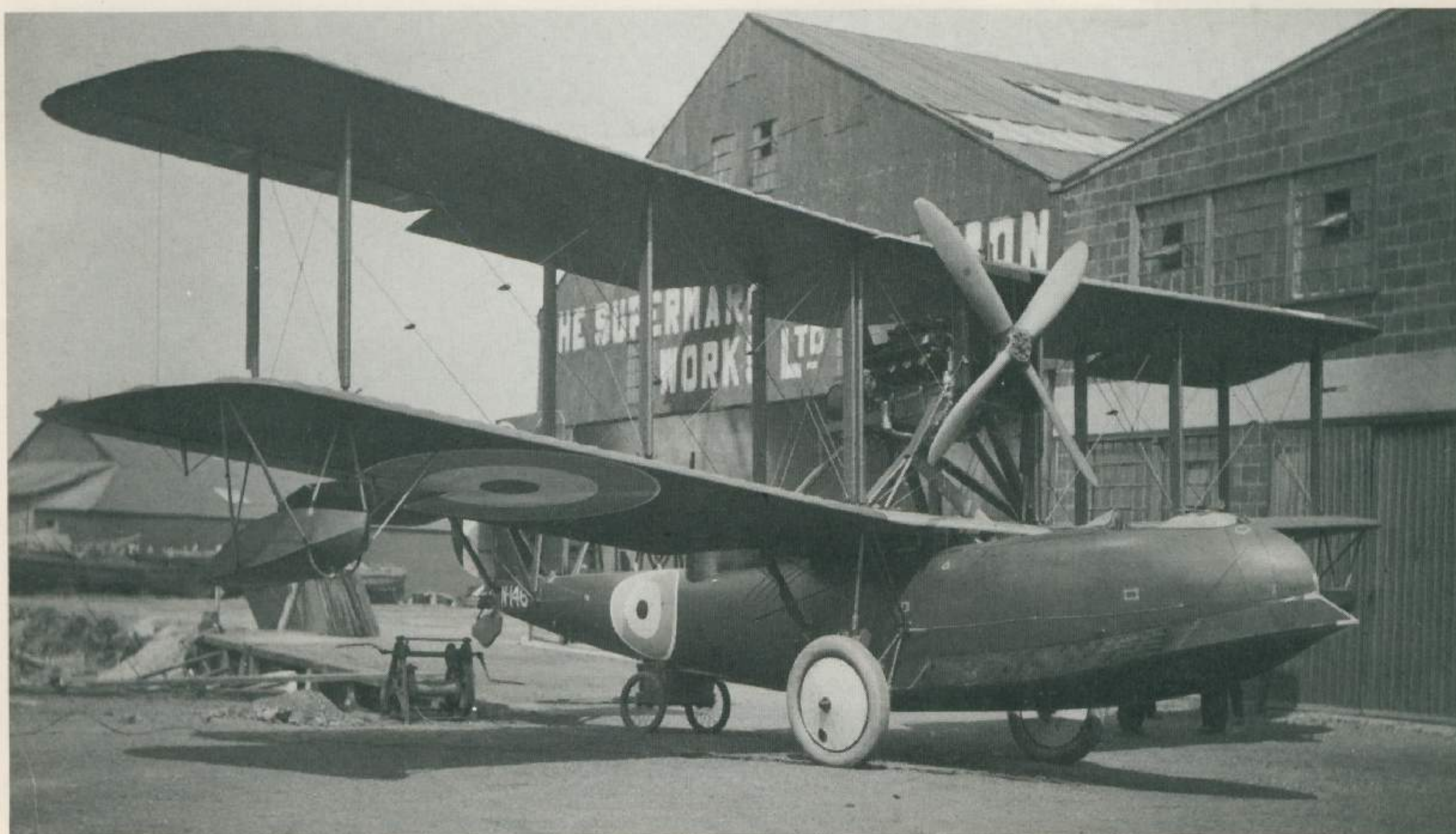
Mother: N146, the Supermarine Seal , the 1921 name for the later military Seagull series. Note the Linton Hope hull form and the simple upward-and-outward (but not fully) retracting main wheels. (Photo: Supermarine via Air-Britain archives)
