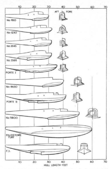
Hulls to the design of John Porte. No complete details are available on the section of the Fury's hull.
