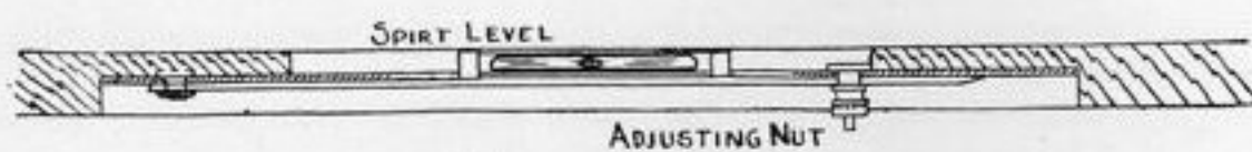
FIG. 5.—ADJUSTABLE LEVEL FOR DIHEDRAL ANGLE.
