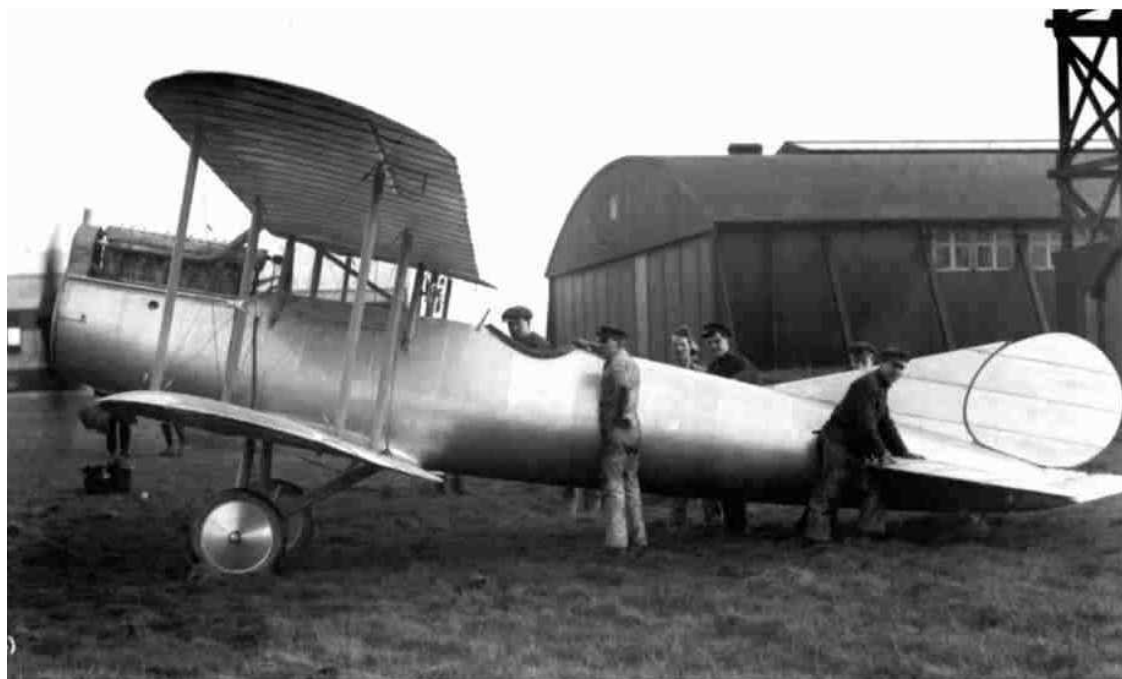
3. Short Bros. photo H 23 (b). The Silver Streak in original single seat form The lower case suffix attached to Short Bros. photographs. (b) in this case, usually indicated that the photograph formed part of a series taken for record purposes before, or sometimes during, the first flight of a newly completed aircraft.
