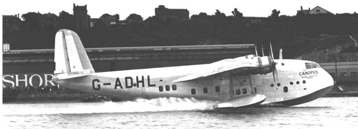
19. Short Bros. photo H.907 (g). 'HL CANOPUS gathering speed for take off on 4 July 1936 before an assembled multitude of spectators. Note the original sprung float arrangement, the un-painted mahogany trim tab, the lack of the servo tab on the rudder and the original position for the owner and port of registration lettering.
