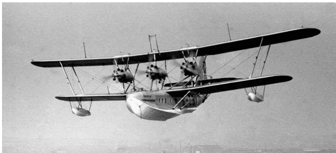
6. Short bros. photo H 243 (j). Short Calcutta G-EBVG over the Medway. The lines of the hull and planing bottom are seen to advantage. 'VG capsized in a storm at Mirabella 28 December 1936.
