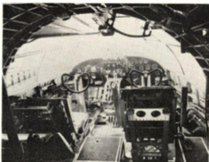
Above, left and right: Canopus cockpit looking aft and showing radio station, pilots' controls and greenhouse.
