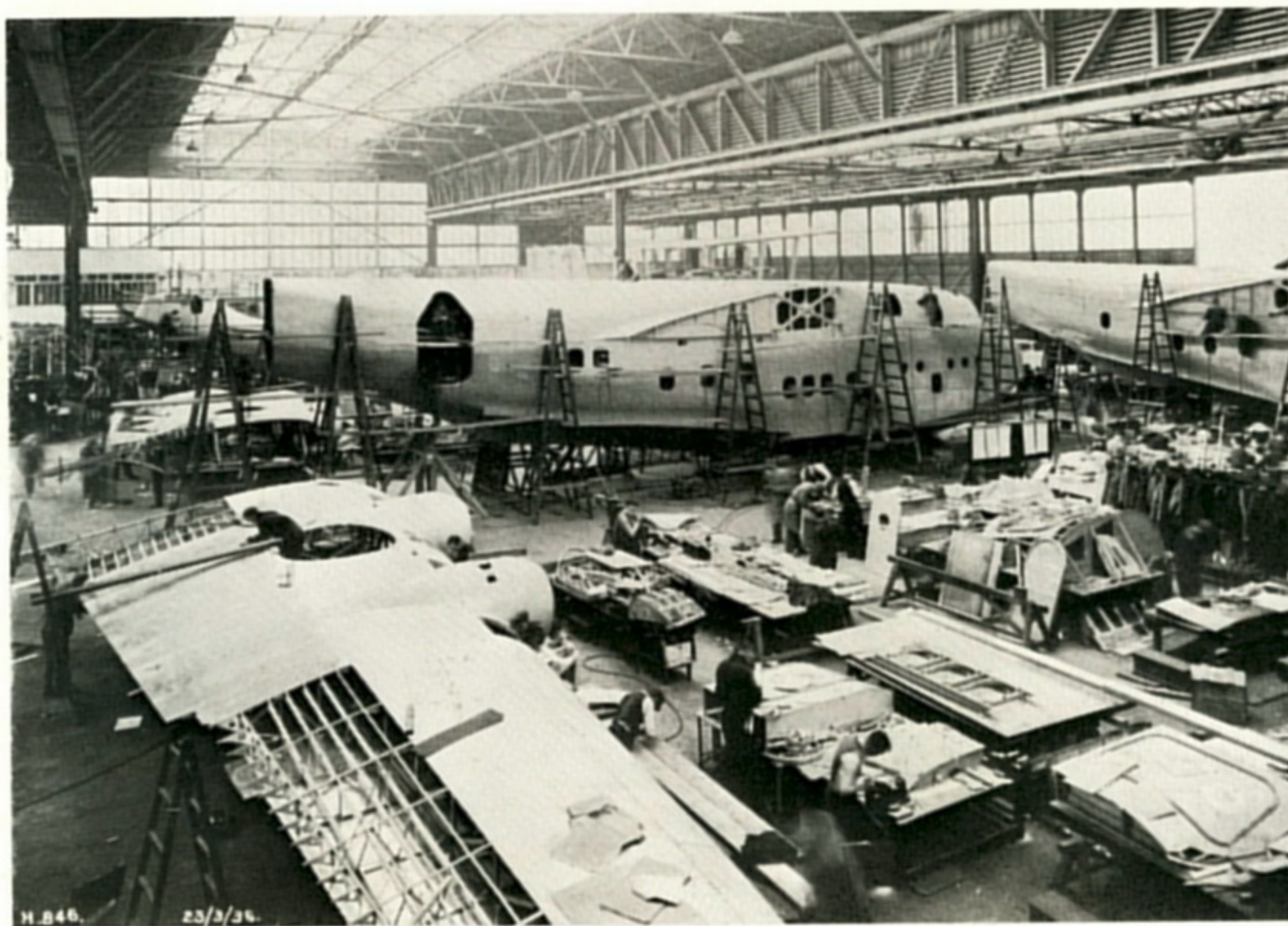
Even this excellent view of activity in the Short works does not do justice to the impressive scene, for it does not include the row of nine towering hulls packed side by side for plating. Incidentally, when a completed boat is moved out on to the slipway there is a clearance of about six inches between the tail and the lintel.
