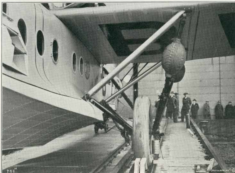
FIG. 57. DETACHABLE LAUNCHING TROLLEY ON PORT SIDE.
