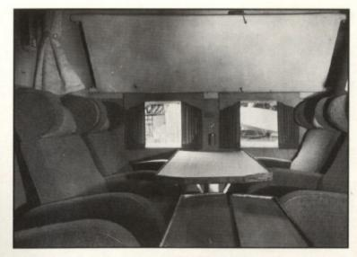
standard. There were three interior layouts: H.1 with 16 passengers on the main deck; H.2 with a promenade deck and H.3 with 24 seats. The Sunderland's front turret fairing was retained — it slid aft — to facilitate mooring. After conversion the 'boats were known as the Hythe class and had names beginning with H. One, G-AGKX, was further modified with faired bows and tailcone and became the sole Sandringham 1,
