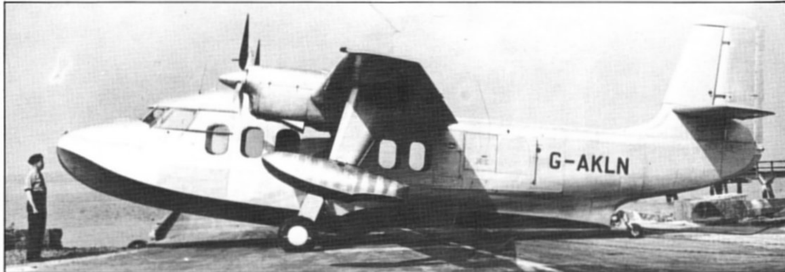
Short Sealand G-AKLN in classic MAEE pose. Every aircraft taken on charge by MAEE was photographed at the head of the slipway, usually with an airman to give scale. MAEE pilots criticised G-AKLN's handling on the water and at take-off while assessing the Sealand in the air-sea rescue role during the autumn of 1950. □ Bill Mortimer
