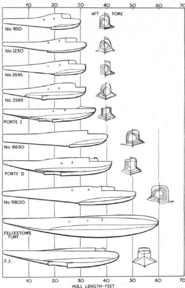
Hulls to the design of John Porte. No complete details are available on the section of the Fury's hull.
