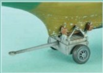
The tail trolley is the early pattern; later versions had double wheels on the single axle
