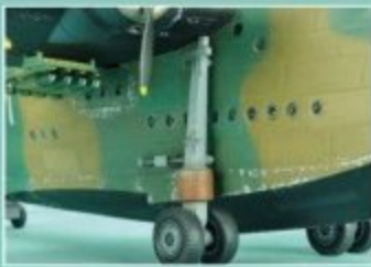
The main undercarriage beaching attachments are huge lumps of angle iron with a cork foot wrapped around them; it's all so agricultural isn't it great?
