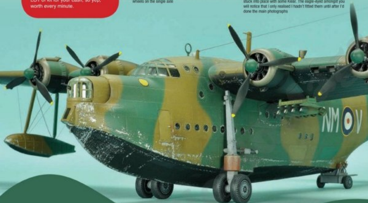
The tail trolley is the early pattern; later versions had double wheels on the single axle
