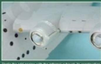
That's the odd engine with the internal exhaust, its construction is different to the other three
